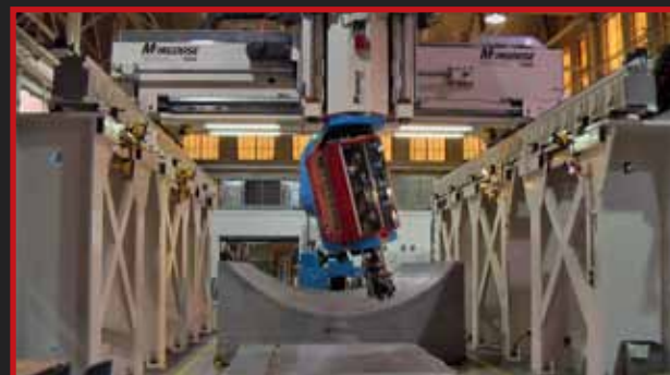
Gantry-crane Fiber Placement.
